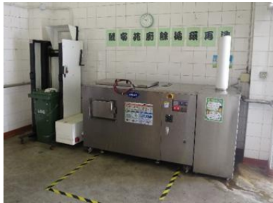
On-site composting machines turn food waste into compost
